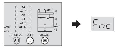
Press the [DRAWER] button several times until the lamp of the drawer in which you placed paper is lit.
